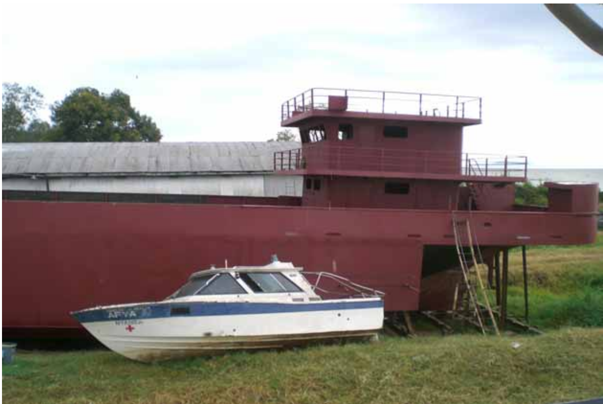
Kavirondo being lengthened on the slipway in Kisumu
