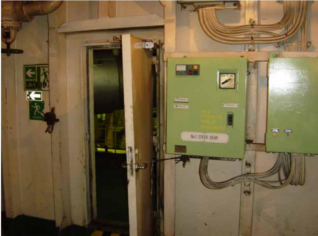
Unfortunately the gagging open of this single fire door can be fatal. The foam system and emergency fire pump are often fitted in the steering flat and in the event of an engine room fire, they would be rendered useless. Where CO<sub>2</sub> is concerned, the steering flat is not a machinery space for the purpose of calculating the volume / amount of gas needed, leaving this door open will have a diluting effect and reduce its effectiveness.
